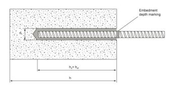
Table A2: Installation details for rebar
